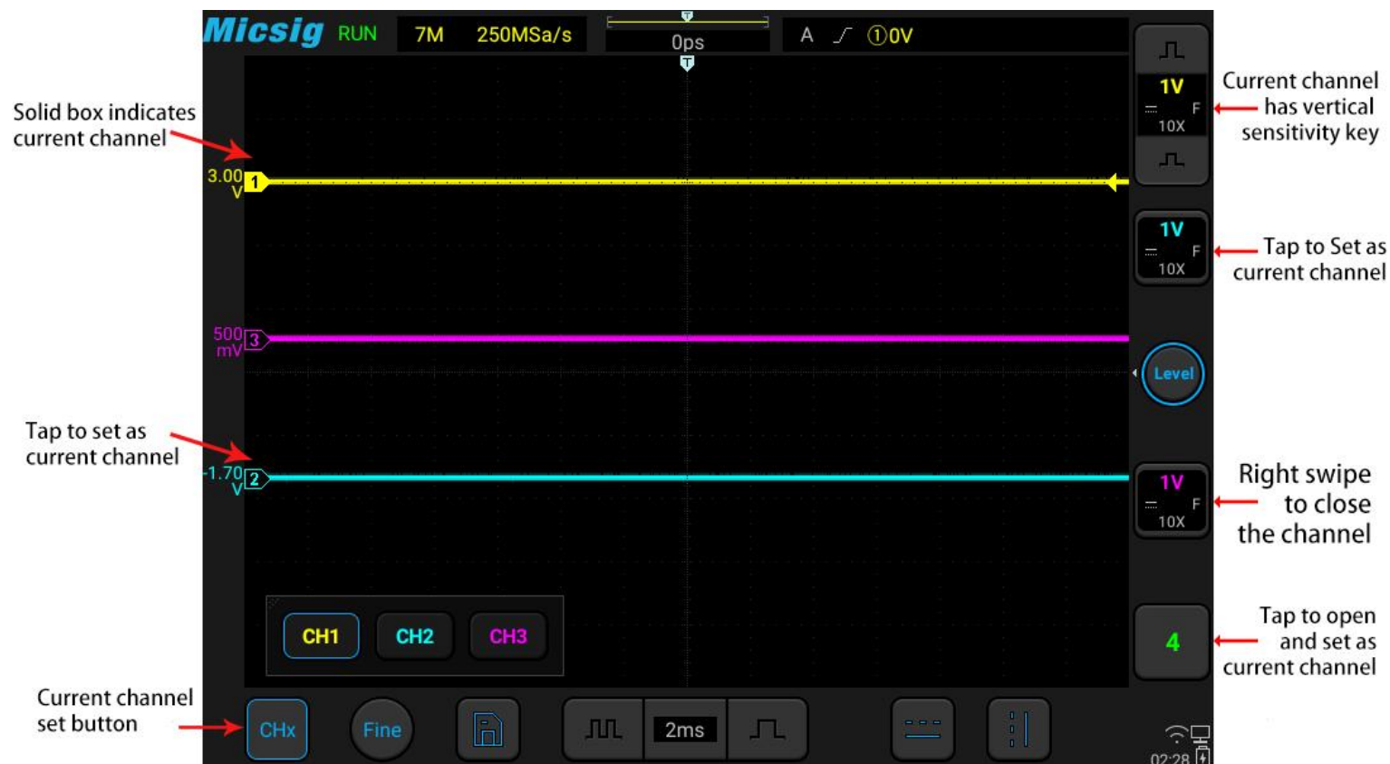
Figure 5-4 Channel Open, Close and Switching
