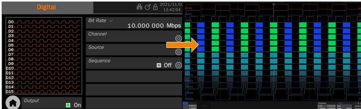
Purchase the corresponding digital bus kit to get 16-channel LVTTTL or LVDS output with a bit rate of 1  $\mu$ bps ~ 1 Gbps. Combine the digital bus with the analog channels to realize mixed-signal outputs.
