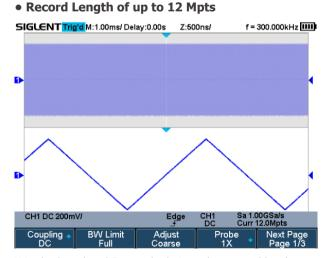
Using hardware-based Zoom technologies and max record length up to 12 Mpts, users can oversample to capture for longer periods at higher resolution and use the zoom feature to see more details within each signal.
