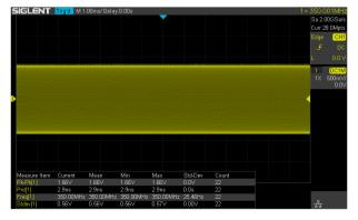
SDS2000X-E can apply automatic measurements on all sampled data points up to 28 Mpts. This ensures the accuracy of measurements while the math co-processor decreases measurement time and increases ease-of-use.
