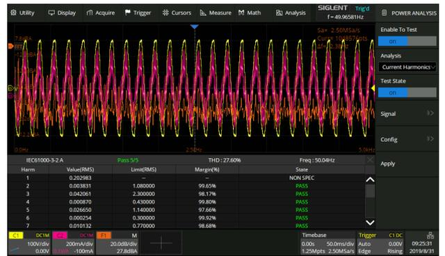
The Power Analysis option provides a full suite of power measurements and analysis, which greatly improve the measurement efficiency in switching power supplies and power devices design.
