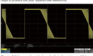
The rise/fall times can be set independently to the minimum of 8.4 ns at any frequency and to the maximum of 22.4 s. The adjustment step is as small as 100 ps.
