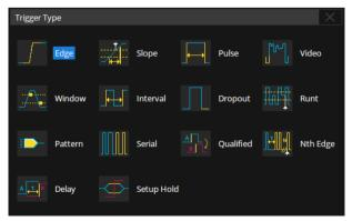
Edge, Slope, Pulse, Video, Windows, Runt, Interval, Dropout, Pattern, Qualified, Nth edge, Setup/hold, Delay and serial trigger
