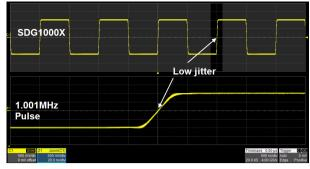
When a Pulse waveform is generated by a common DDS generator, there will be a one-clock-jitter if the sampling rate is not an integer-related multiple of the output frequency. SDG1000X EasyPulse technology successfully overcomes this weakness in DDS designs and helps to produce low jitter Pulse waveforms.
