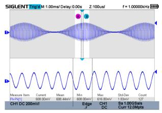
Through Gate and Zoom measurement, the user can specify an arbitrary interval of waveform data analysis and statistics. This helps avoid measurement errors that can be caused by invalid or extraneous data, greatly enhancing the measurements' validity and flexibility.
