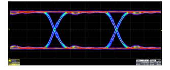
\*CH1:PRBS.ON.50Ω CH2:PRBS.ON.50Ω 122.880 000Mbps Bit Rate Amplitude 800.0mVpp Offset 850.0mVdc Length PRBS-30 Rise/Fall 2.0ns Load 50 Ω ON **P** = Output Differential LVTTL LVCOMS TTL/CMOS LVDS ECL LVPECL **ON**
