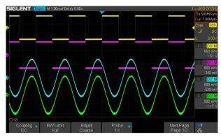
The four channel series has two 1 GSa/s ADC chips (channel 1 and 2 share one, channel 3 and 4 share another), so that each channel can achieve sample rates up to 500 MSa/s and work on bandwidths of 200 MHz when all channels are enabled.
