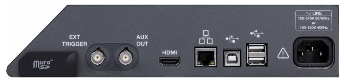
USB Host 3.0 x2, USB Host 2.0 x2, USB Device 2.0 (USBTMC) x1, LAN (VXI-11/Telnet/Socket) x1, micro SD card x1, Auxiliary output (Pass/Fail, Trigger Out)x1 and HDMI x1
