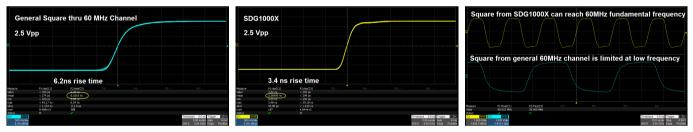
Benefitting from a special square-wave generating circuitry, the Square from the SDG1000X breaks the 60 MHz bandwidth barrier, reaching rise/fall times of less than 4.2 ns, and frequencies up to 60 MHz.
