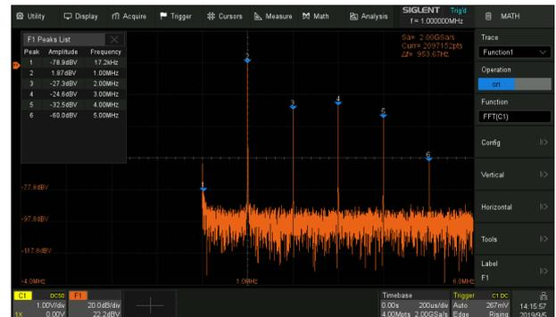
Hardware accelerated FFT up to 2 Mpts. This provides high frequency resolution with fast refresh rate. The FFT function also supports a variety of window functions so that it can adapt to different spectrum measurement needs. Three modes (Normal, Average and Max hold) can satisfy different requirements for observing the power spectrum. Auto peak detection and markers are supported.
