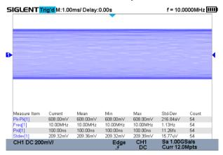
SHS800X/SHS1000X series can measure all sampled data points up to 12 Mpts. This ensures the accuracy of measurements while the math coprocessor decreases measurement time and increases ease-of-use.
