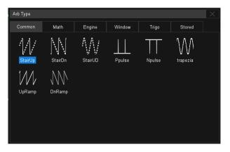
The built-in waveform generator can output waveforms with up to 50 MHz frequency and  $\pm 3$  V amplitude. Six basic waveforms together with multiple types of predefined waveforms and as user defined arbitrary waveforms are supported.
