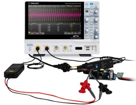
The Power Analysis option provides a full suite of power measurements and analysis, which greatly improve the measurement efficiency in switching power supplies and power devices design
