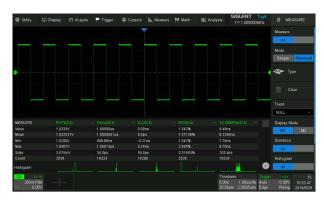
Parameter measurements includes 4 categories: Vertical, Horizontal, Miscellaneous and Channel Delay providing a total of 50+ different types of measurements. Measurements can be performed within a specified gate period. Measurements on Math, Reference and History frames are supported.
