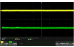
Low noise floor: Only 70  $\mu\text{Vrms}$  at 500 MHz bandwidth
