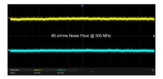
Low noise floor: Only 80  $\mu V$  rms at 500 MHz bandwidth.
