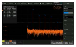
Hardware-accelerated FFT supports up to 2 Mpts operation. This provides high-frequency resolution with a fast refresh rate. The FFT function also supports a variety of window functions so that it can adapt to different spectrum measurement needs. Three modes (Normal, Average, and Max hold) can satisfy different requirements for observing the power spectrum. Auto peak detection and markers are supported
