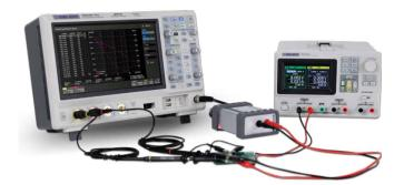
The SDS2000X Plus can control the built-in waveform generator or any stand-alone SIGLENT SDG device to scan the amplitude and phase response over frequency of passive or active circuits. The data is presented as Bode Plot. This makes it possible to replace expensive network analyzers in less demanding applications.
