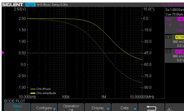
SDS2000X-E can control the USB AWG module or an independent SIGLENT SDG instrument, scan a circuits amplitude and phase frequency response, and display the data as a Bode Plot. It can also show the result lists, and export the data to a USB disk.
