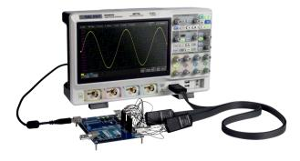
Four analog channels plus 16 digital channels enable users to acquire and trigger on the waveforms then analyze the pattern, simultaneously with one instrument • Built -in 25 MHz Function / Arbitrary Waveform Generator (Optional)
