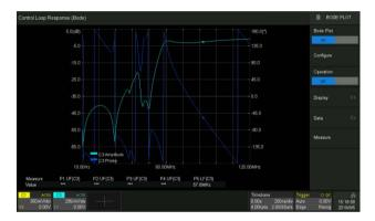
The SDS5000X can control the USB AWG module or a stand-alone SIGLENT SDG generator, to scan the amplitude and phase frequency response of the DUT, and display the data as a Bode Plot. This makes it possible to replace expensive network analyzer in some applications.
