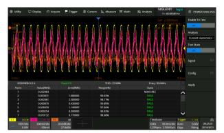
The Power Analysis option provides a full suite of power measurements and analysis, thus improving the efficiency of measurement in switching power supplies and power device designs.
