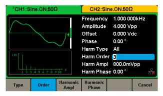
Up to 10 harmonics may be generated. Amplitude and phase of each harmonic can be set independently.
