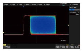
Segmented memory collection will store the waveform into multiple memory segments (up to 100,000) and each segment will store a triggered waveform as well the dead time information. The dead time between segments can be as small as 2  $\mu$ s. All of the segments can be played back using the History function
