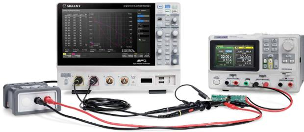
The oscilloscope can control the built-in waveform generator or a stand-alone SIGLENT generator, to scan the amplitude and phase-frequency response of the DUT, and display the data as a Bode Plot. This makes it possible to replace expensive network analyzers in some applications
