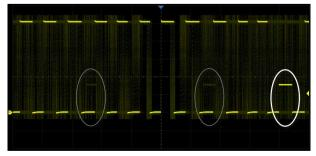
With a waveform update rate of up to 100,000 wfm/s, the oscilloscope can easily capture unusual or low-probability events. In Sequence mode, the waveform capture rate can reach 500,000 wfm/s
