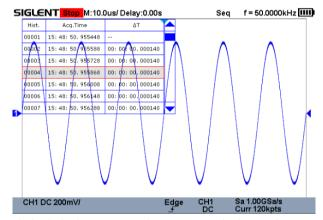
Playback the latest triggered events using the history function. Segmented memory collection will store trigger events into multiple (Up to 80,000) memory segments, each segment will store triggered waveforms and timestamps for each frame.
