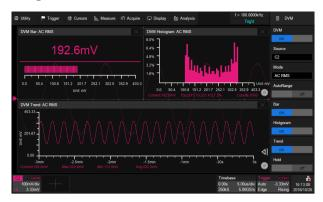
4-digit voltmeter and 7-digit frequency counter. Any analog channel can be selected as a source. Bar, Histogram and Trend diagrams are supported
