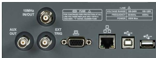
USB Host, USB Device (USBTMC), LAN (VXI-11, telnet, socket, web), Pass / Fail, Trigger Out, 10 MHz In / Out and VGA output
