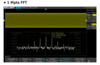
The new math co-processor enables FFT analysis of incoming signals using up to 1 million samples per waveform. This provides high frequency resolution with a fast refresh rate. The FFT function also supports a variety of window functions so that it can adapt to different spectrum measurement needs.
