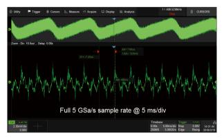
Using hardware-based Zoom technique and record length of up to 250 Mpts, users are able to select a slower timebase without compromising the sampling rate, and then quickly zoom in to focus on the area of interest
