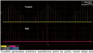
point so that it can reconstruct all the details of the waveform as defined.
