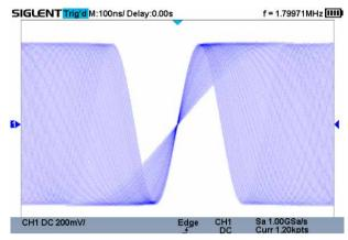
SPO display technology provides fast refresh rates. The resulting intensity-graded trace is brighter for events that occur with more frequency and dims when the events occur with less frequency.
