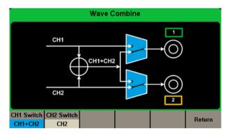
Capable of combining the waveforms of 2 channels from internal, providing more flexible tools to generate complex waveforms.
