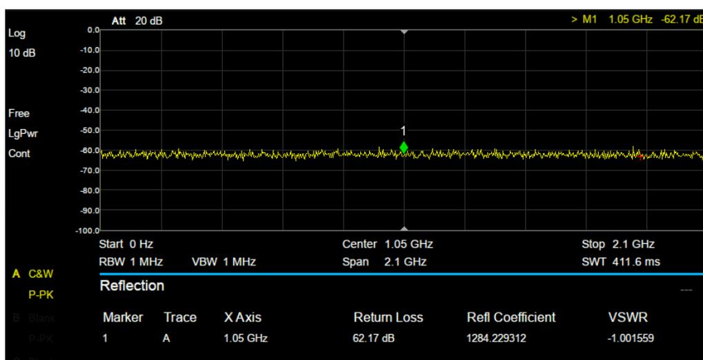
Figure 2-13 Reflection measurement
