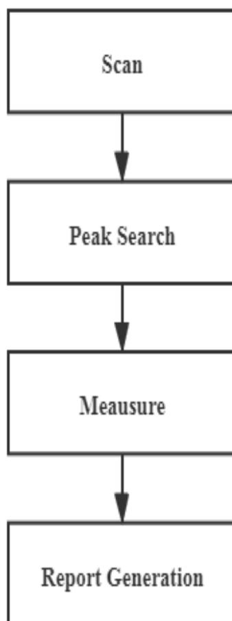
Figure 7-2 CISPR-recommended EMI test flow
