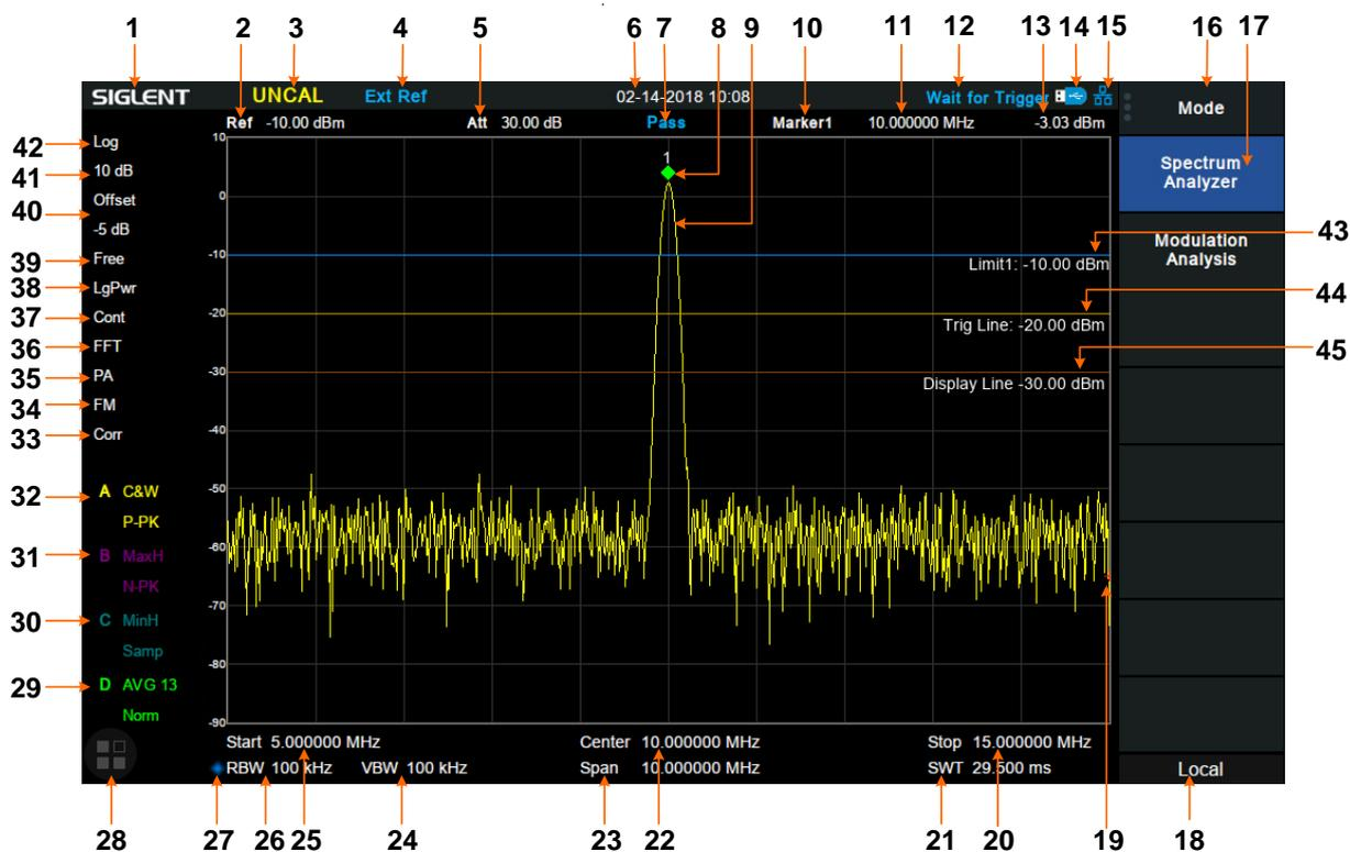
Figure 1-12 User Interface of spectrum analyzer mode
