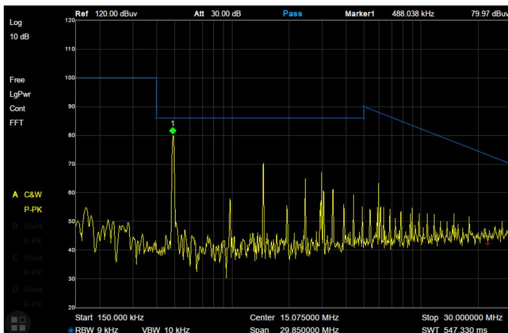
Figure 2-4 Logarithmic X Scale
