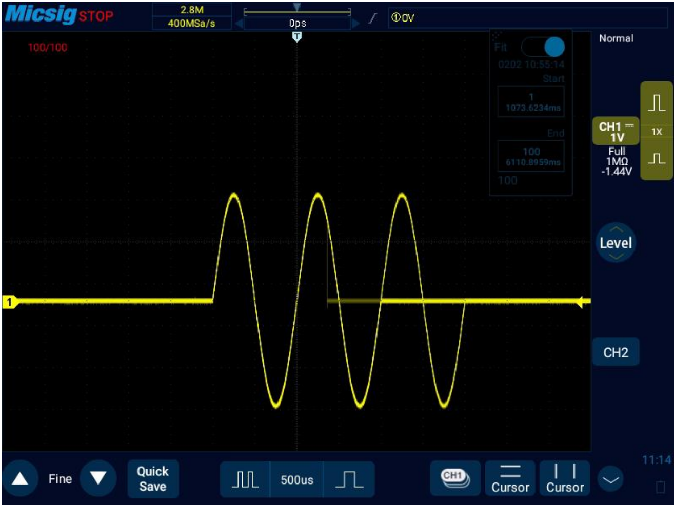
Figure 11-13 Segmented storage fitting view
