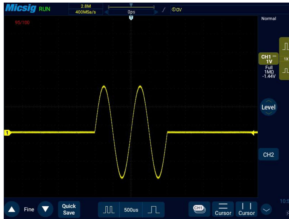
Figure 11-11 Segmented memory waveform acquisition
