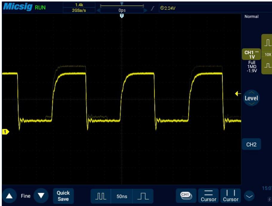
Figure 6-3 Abnormal Signal in Periodic Signals
