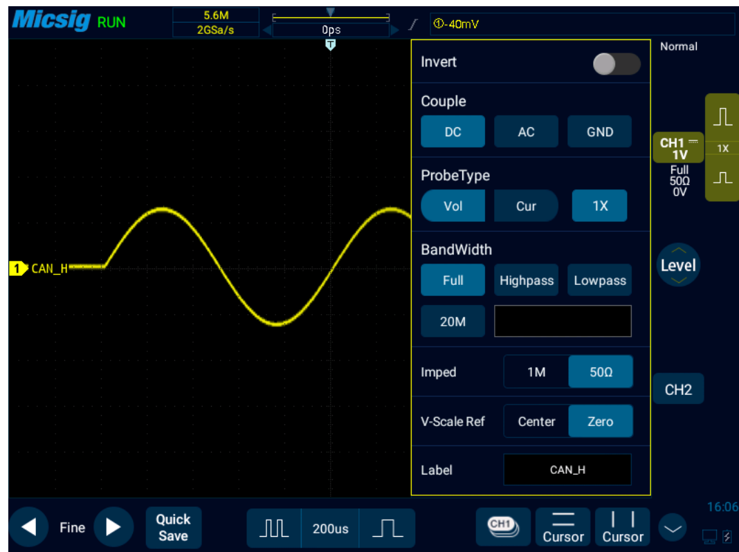
Figure 5-16 Channel Input impedance
