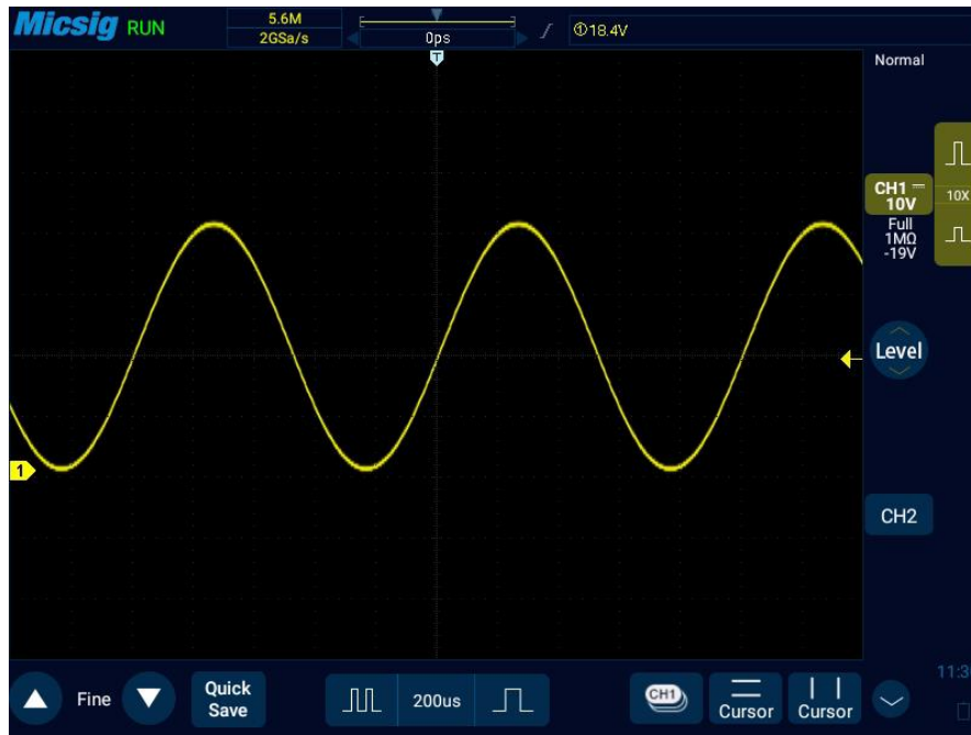
Figure 6-1 Stably Displayed Periodic Signal
