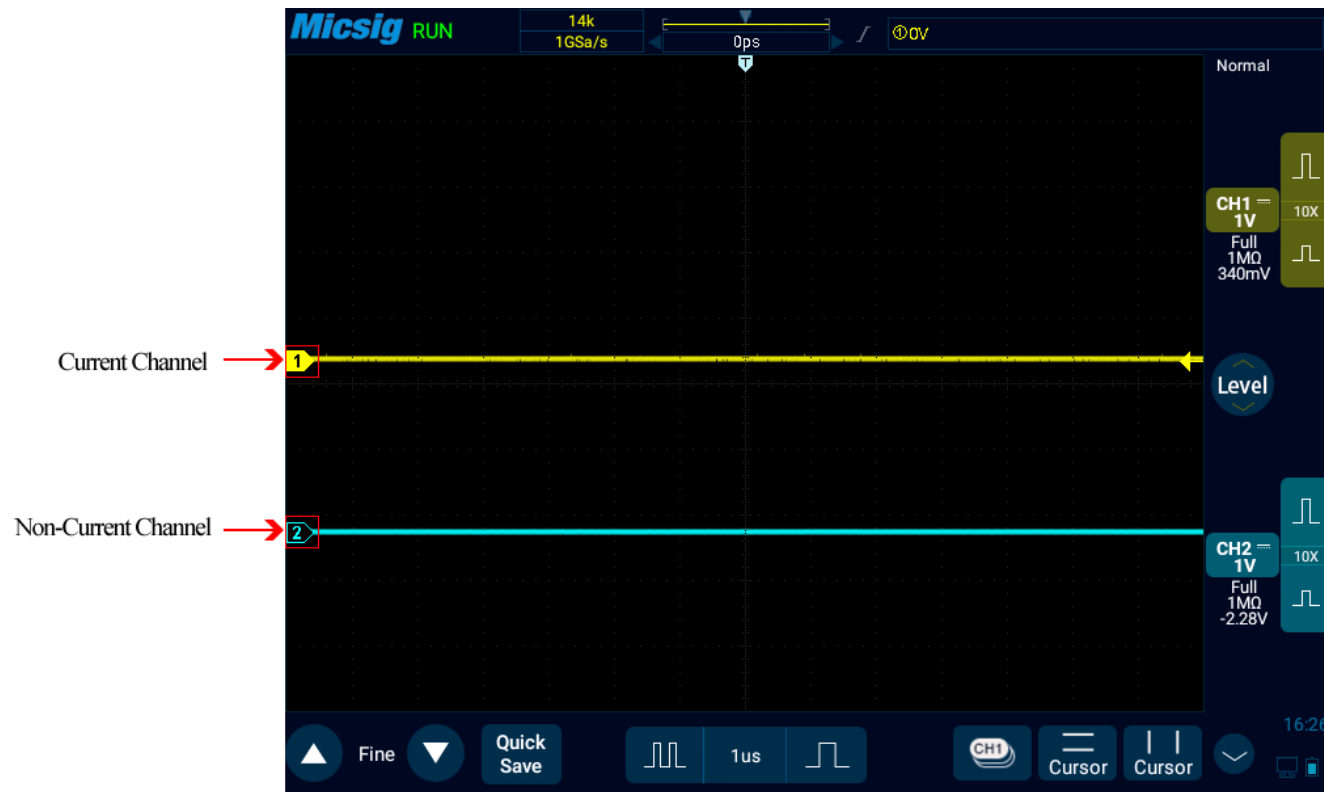
Figure 5-2 Current Channel and Non-Current Channel
