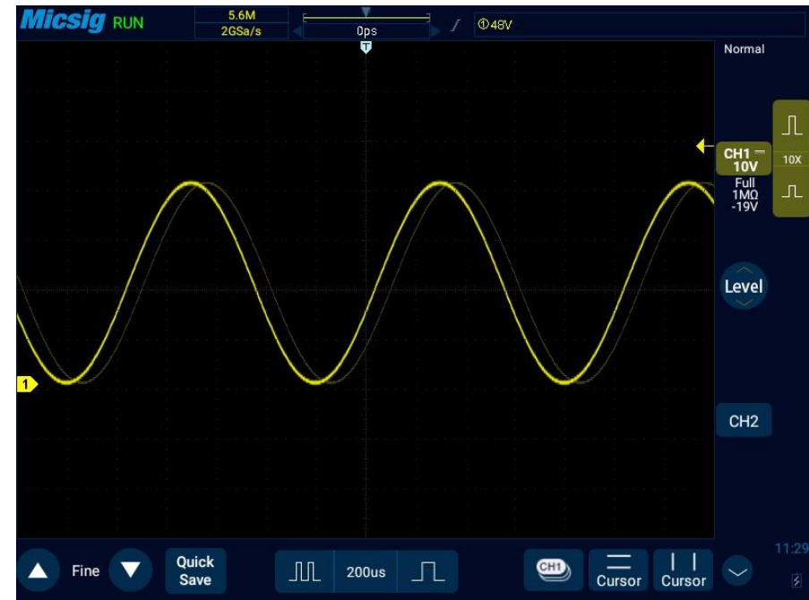
Figure 6-2 Non-Stably Displayed Periodic Signal
