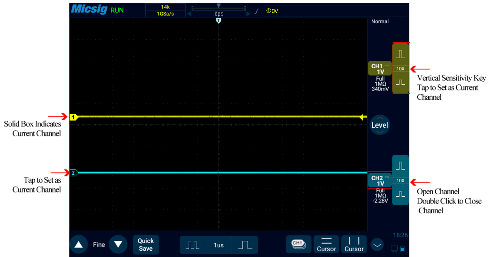
Figure 5-4 Channel Open, Close and Switching
