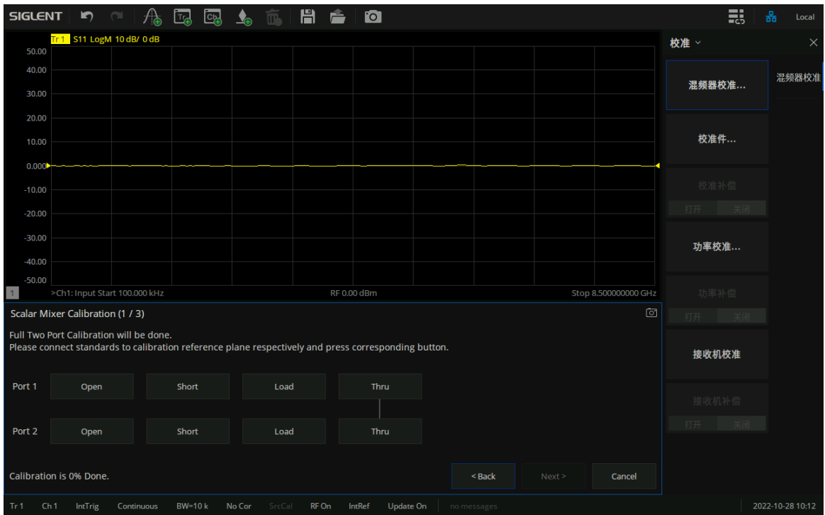
Figure 8-8 The interface of Scalar Mixer Calibration
