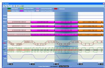
Figure 5: MHL Bus viewer with Physical layer waveforms
