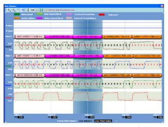
Figure 4: HDMI Bus viewer with Physical layer waveforms
