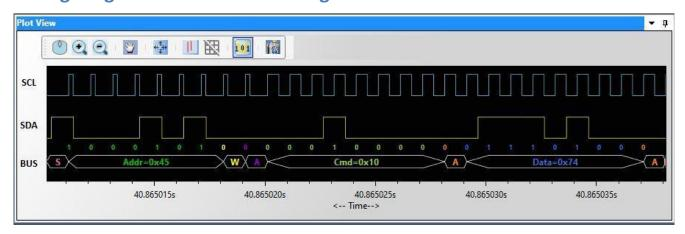
The timing view provides the plot of SCL and SDA signals with a bus diagram. Overlaying of Protocol bits on the digital timing waveform will help easy debugging of Protocol decoded data. Cursor and Zoom features will make it convenient to analyze Protocol in the timing diagram for any timing errors.
