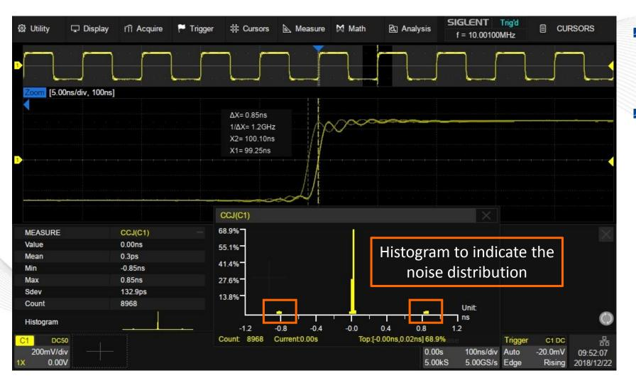
Measure the jitter of a 10.001 MHz signal generated by DDS technology.
