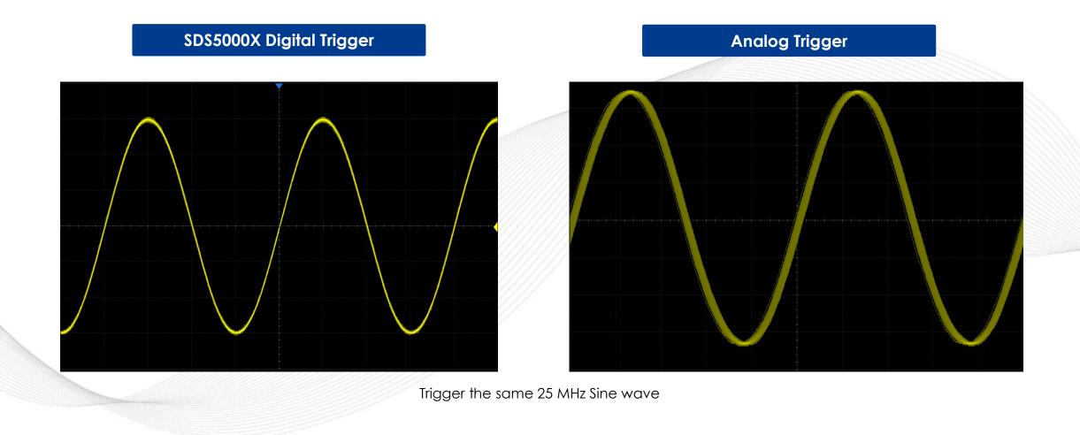
Unique digital trigger system: higher trigger sensitivity, lower trigger jitter (less than 100 ps)
