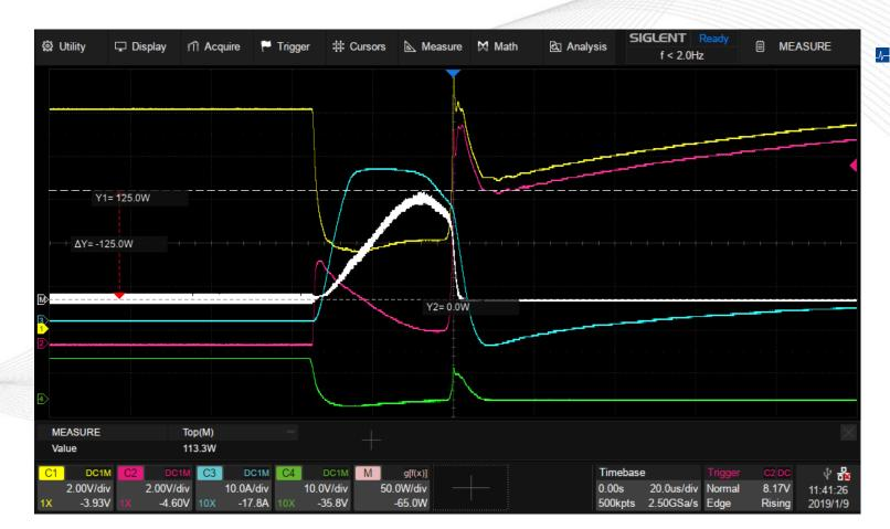
Use a differential probe to measure V<sub>DS</sub> then perform an integral on power to calculate the energy generated when MOSFET is powered on
