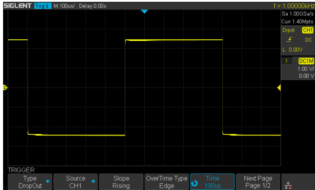
Figure 38 Edge Dropout Trigger
