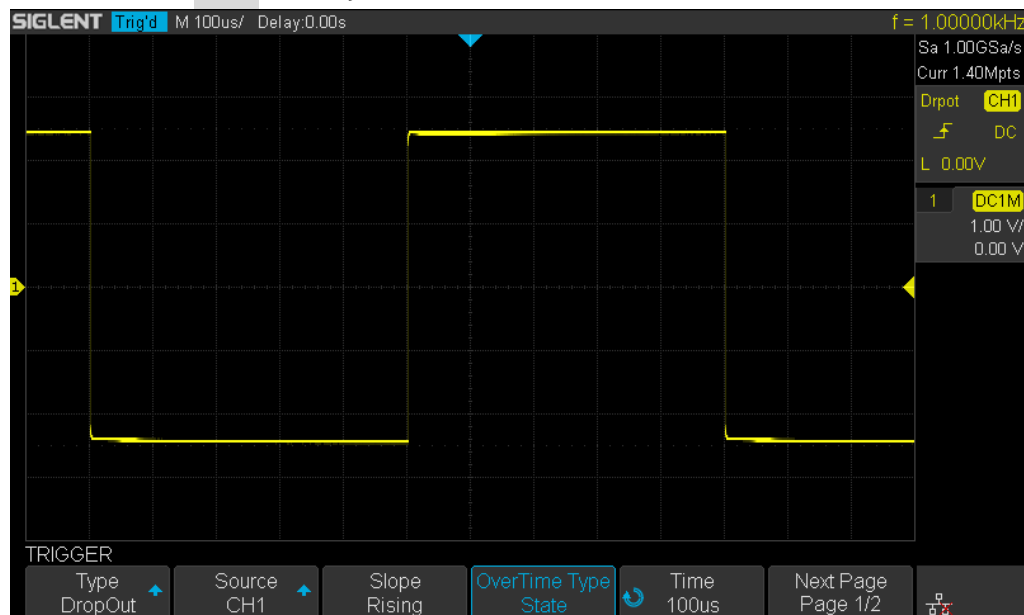
Figure 39 State Dropout Trigger
