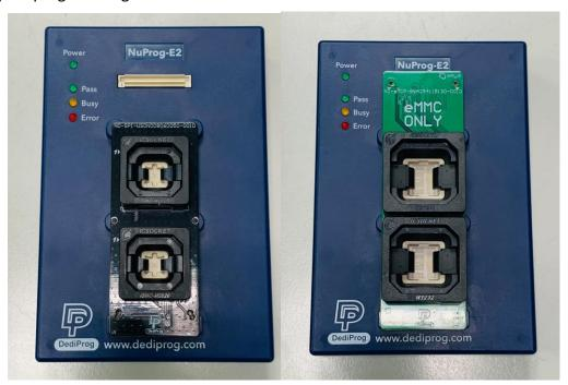
NuProg-E2 can share the socket with NuProgPlus, and NuProg-E2 only supports the upper socket of the Dual Socket.
