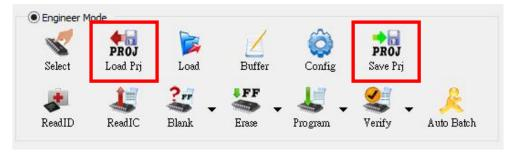
Name the project file (\*.npprj), once the user click ok, a window will appear for the user to set up the password for production management. If the user has set the password, then it will be requested when loading the project in the production mode. If not, then it will load the file directly.
