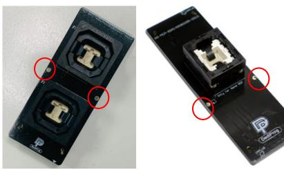
Install the socket adaptor according to the below figure. If the connections are normal, then it is ready for programming.
