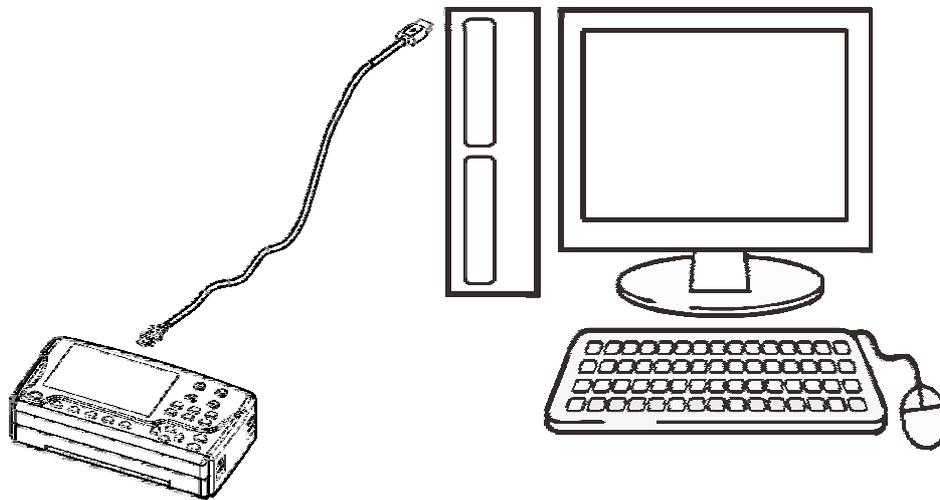
1. Connect one end of the 9803 USB communication cable to the personal computer and the other end to the PC interface above the HT3554.
