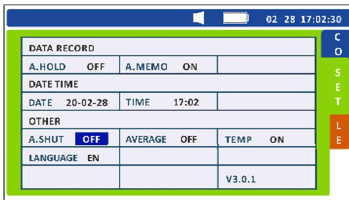
Press [ENTER] to select the automatic shutdown function, and press the left and right keys to switch OFF, ON. Press [ENTER] again to complete. Press [ESC] to return to the measurement interface.
