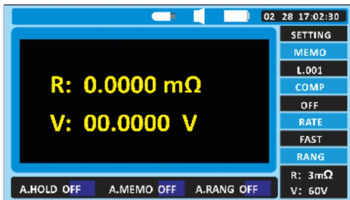
2. When the cable is connected, USB small icon appears in the status bar above the tester, and the 3554 DISK is found on the computer.
