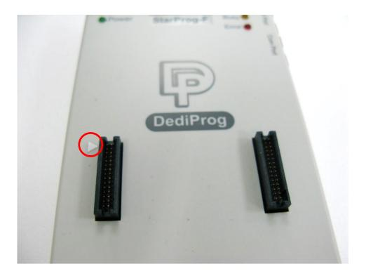
2. Ensure triangles both on the socket and ProgMaster are alignment. Shown as below.
