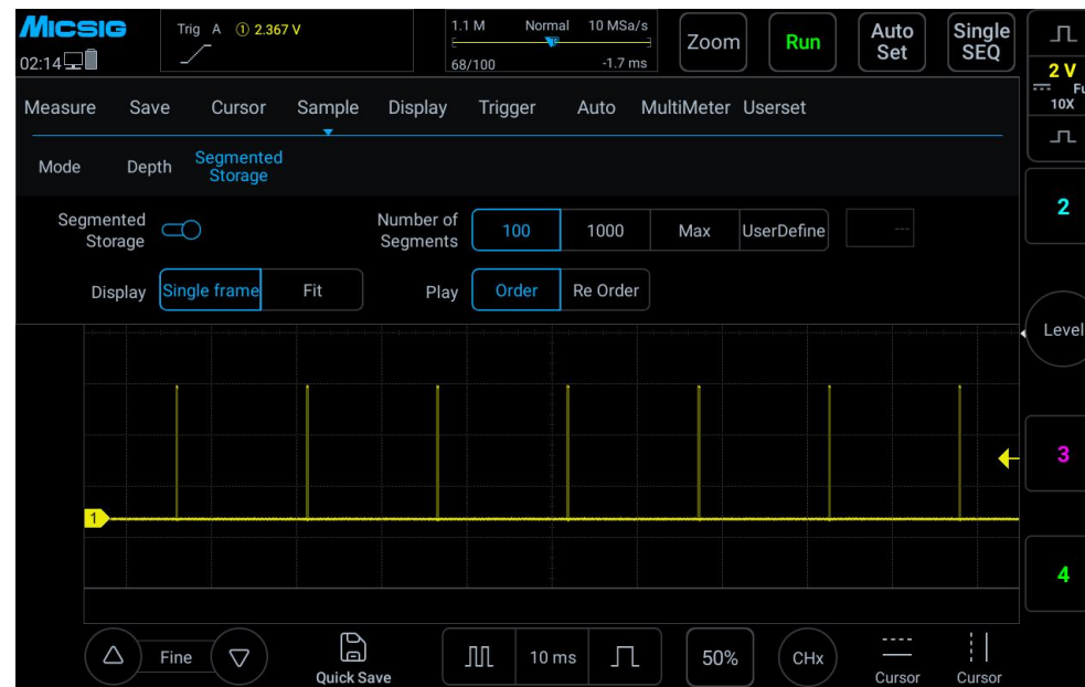
Figure 13-11 Segmented storage waveform acquisition
