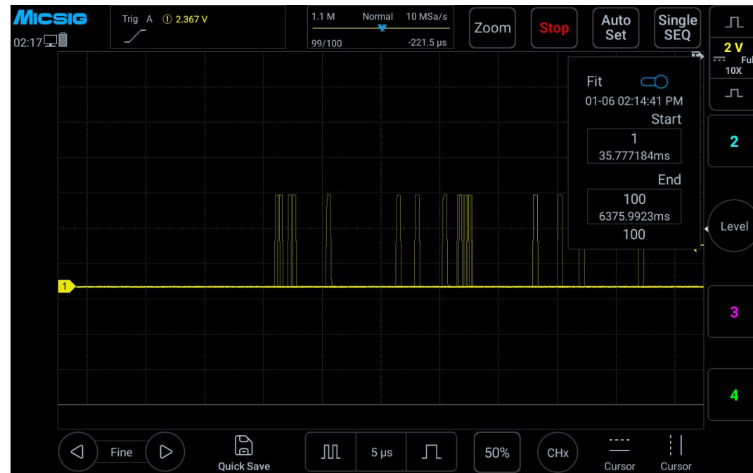
Figure 13-13 Segmented storage fitting view
