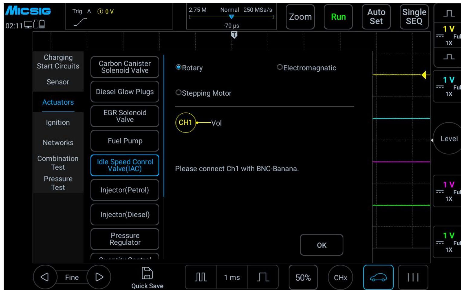
Figure 3-31 Idle speed control valve test
