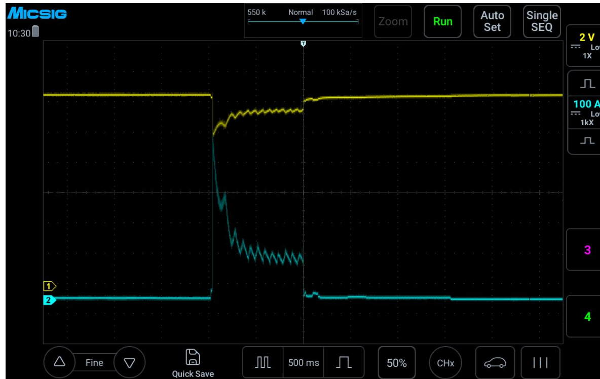
Figure 3-7 Starting voltage and current
