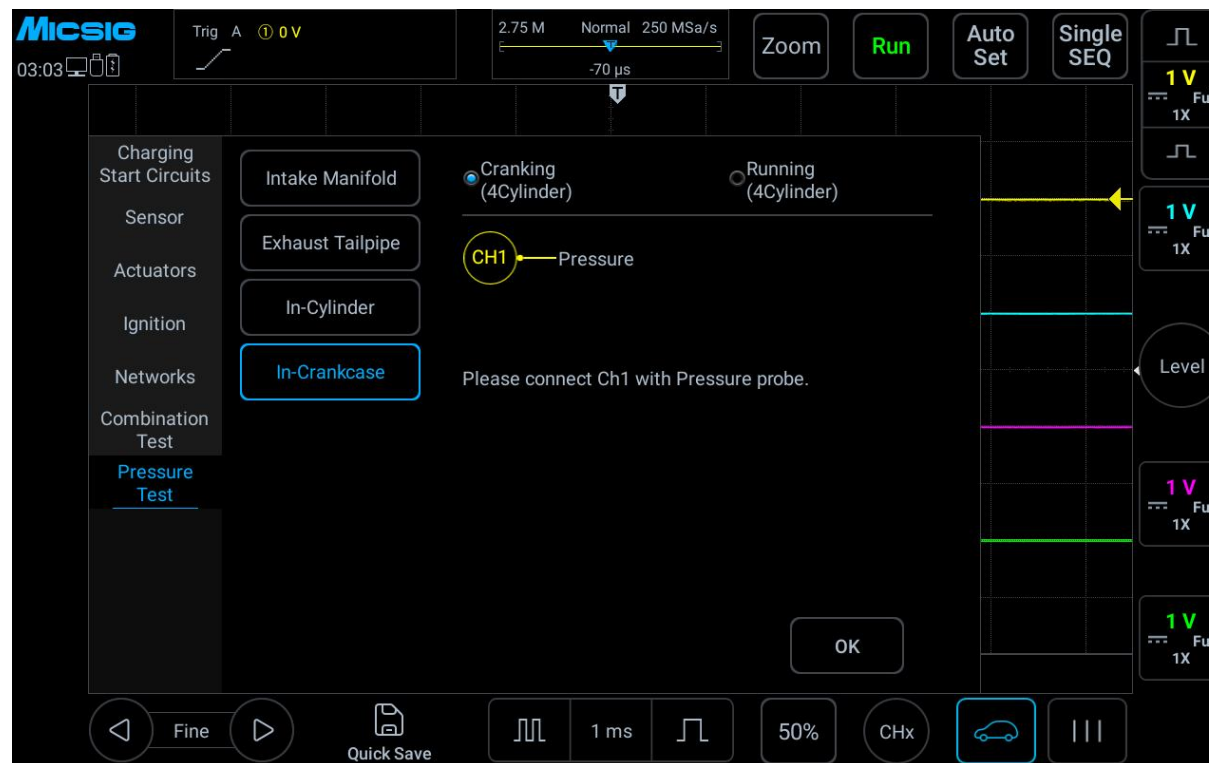
Figure 3-57 In-Crankcase Pressure Test
