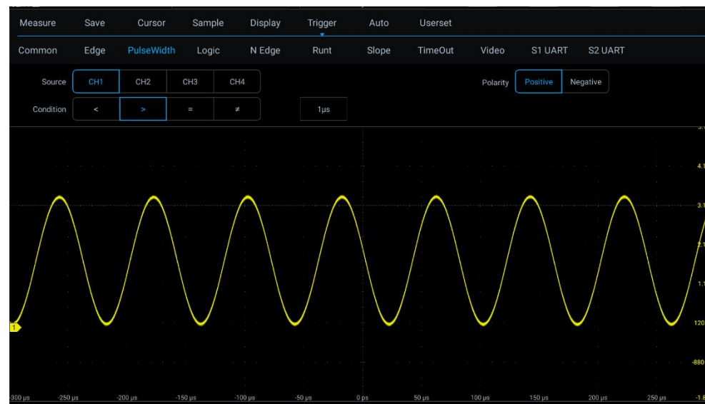
Figure 7-14 Pulse Width Trigger Setting Menu
