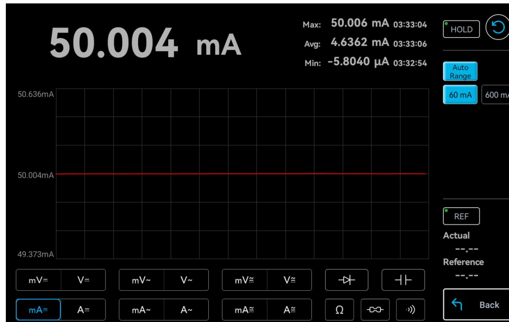
Figure 9-12 DC Current Measurement (mA)
