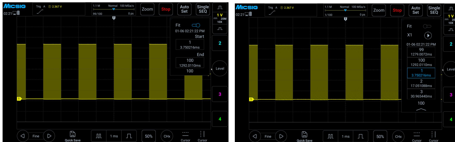
Figure 13-15 View after segment collection is completed
