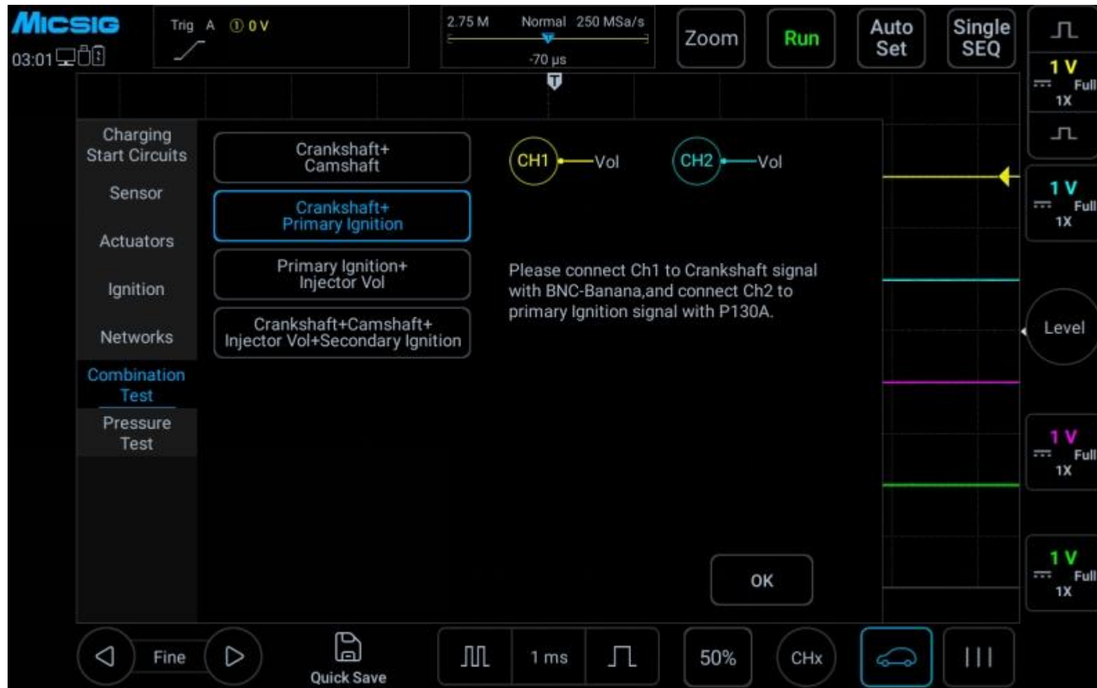
Figure 3-51 Crankshaft + Primary ignition test
