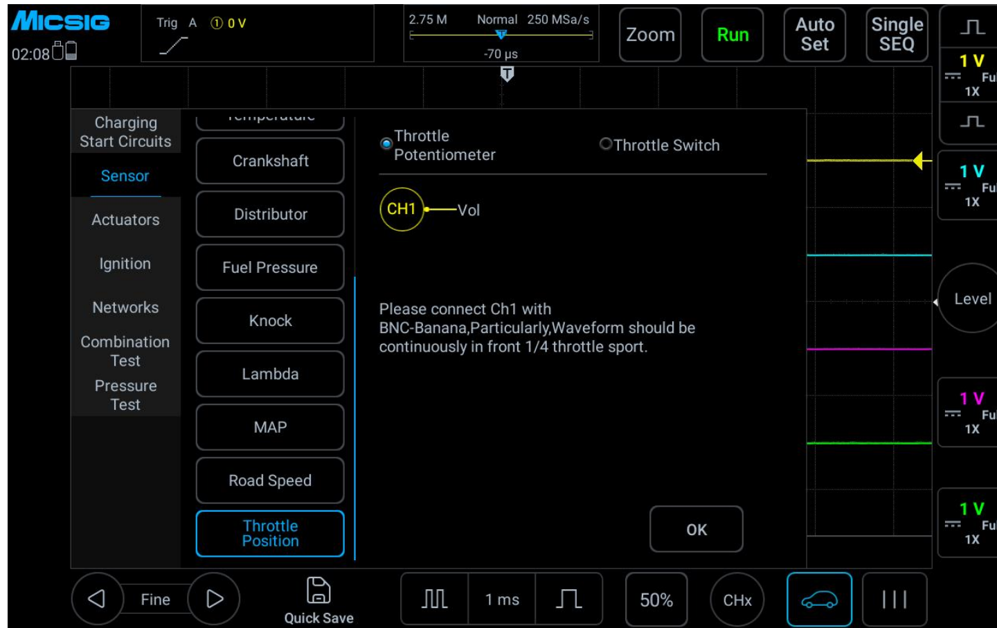
Figure 3-24 Throttle Position Sensor test
