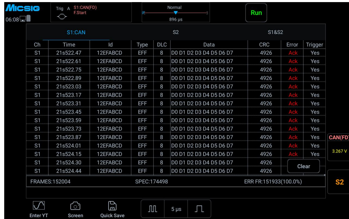
Figure 14-17 CAN bus decode in Text mode
