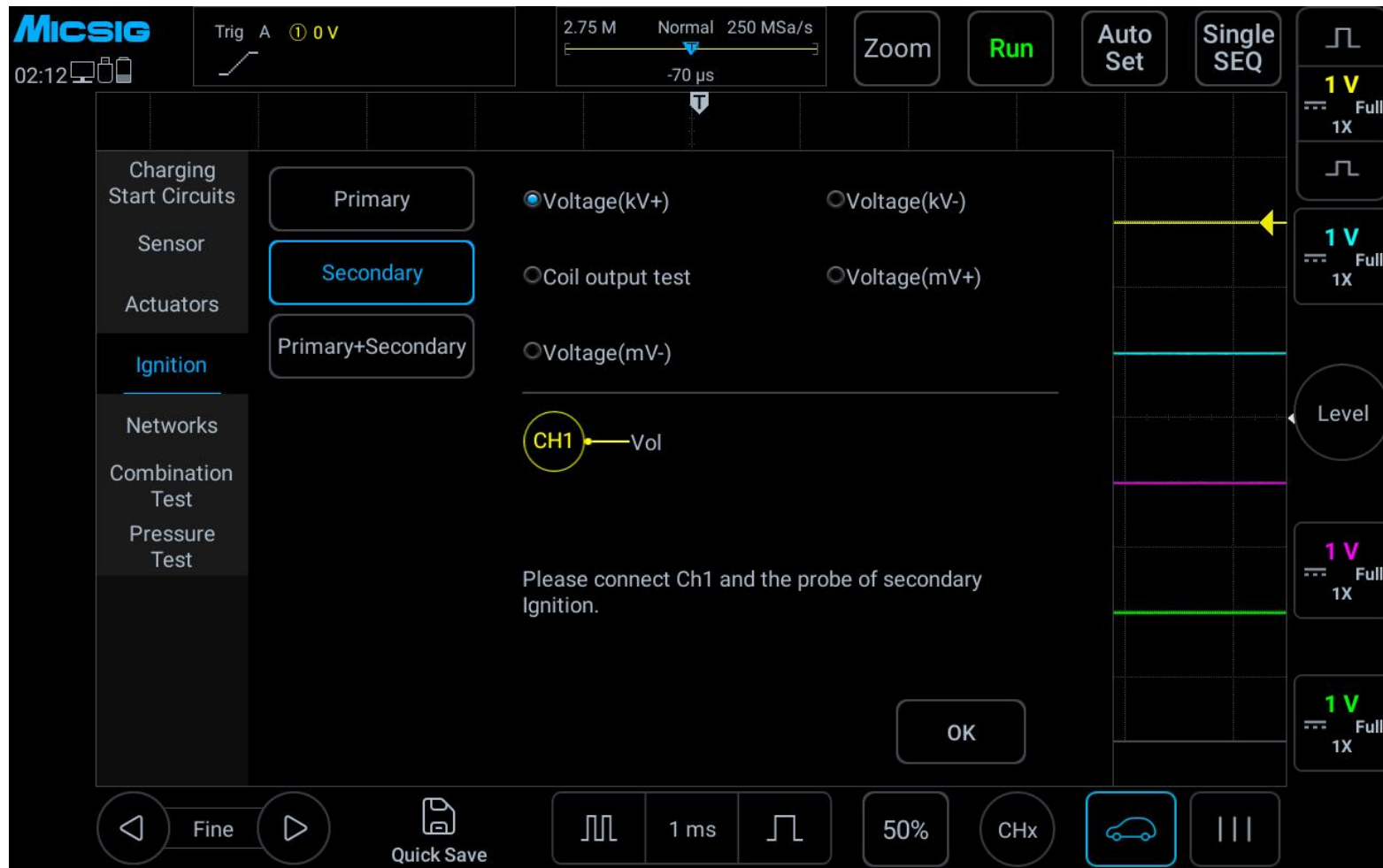
Figure 3-42 Secondary ignition test
