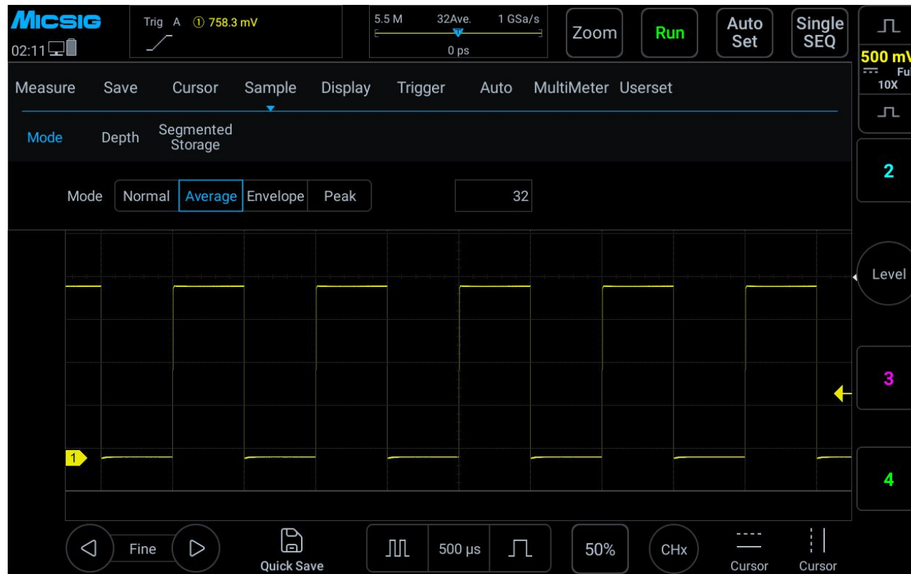
Figure 13-5 The waveform after selecting the average sampling mode, with the average number being 16.
