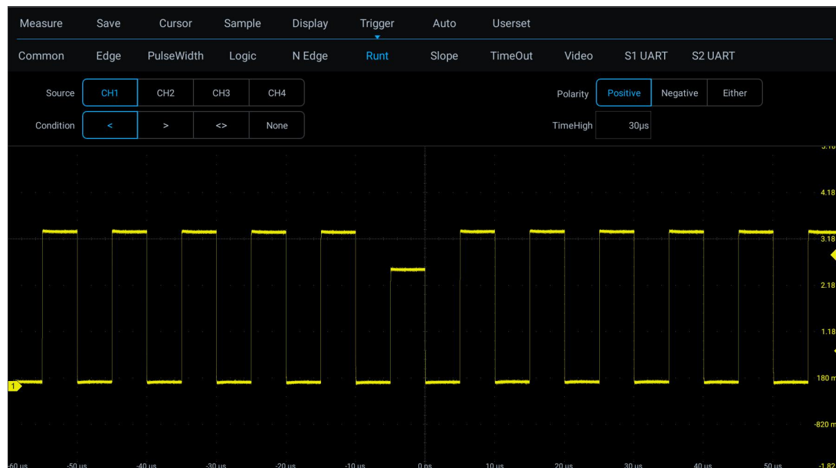
Figure 7-25 Runt Trigger Setting Menu
