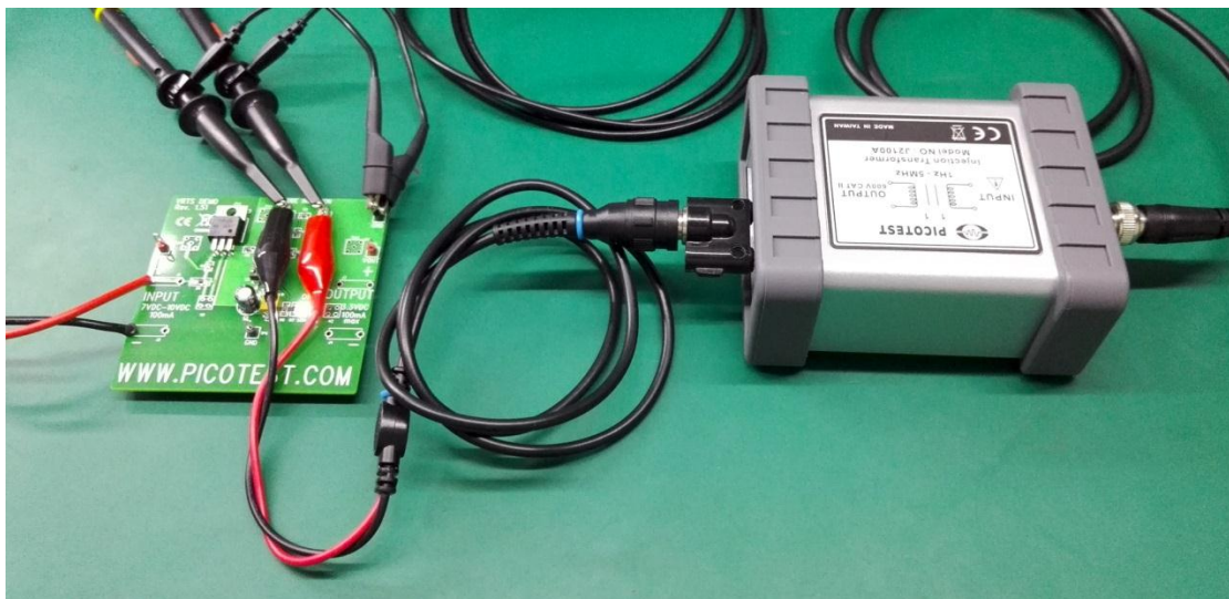
Figure 9 Probe and Transformer Connections in the Actual Circuit
